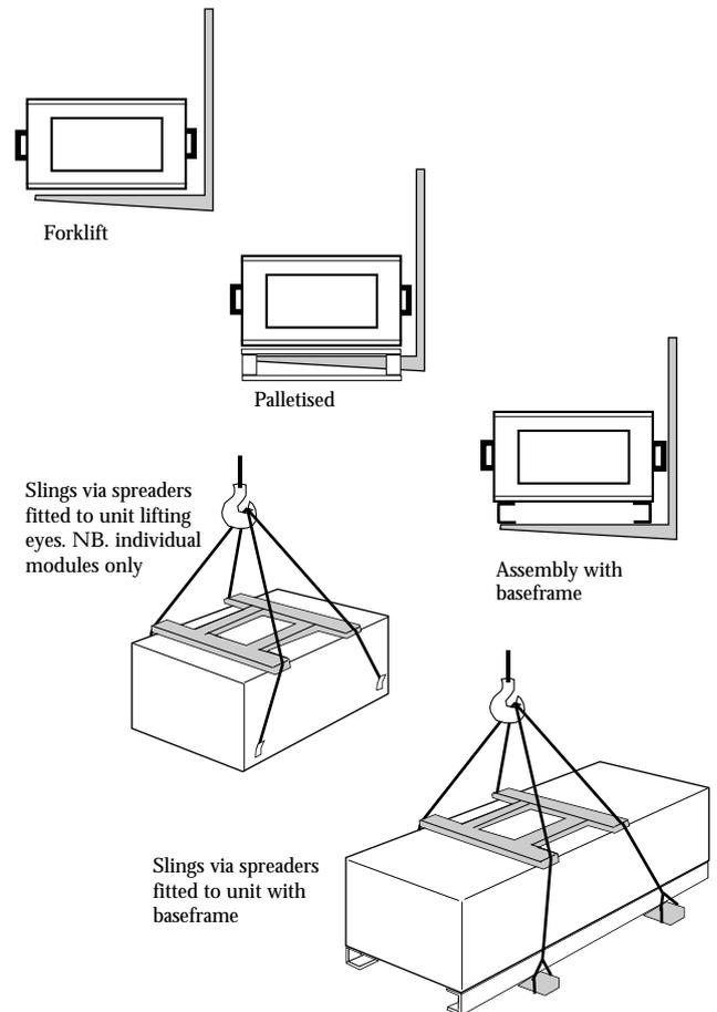
Fig. 3 Lifting and moving the unit.
