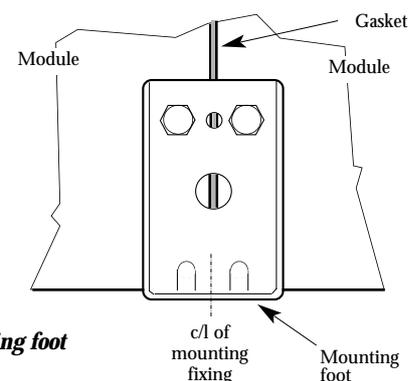
Fig. 5 The mounting foot
