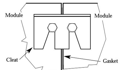
Fig. 4 Fitting a cleat
