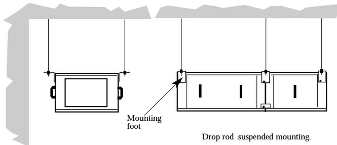
Note: Spacing of supports coincides with module length
