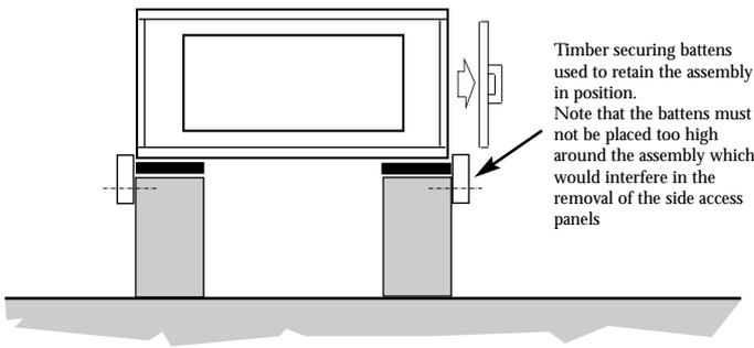
**Fig. 6 Simple builders upstand mounting assembly.**
