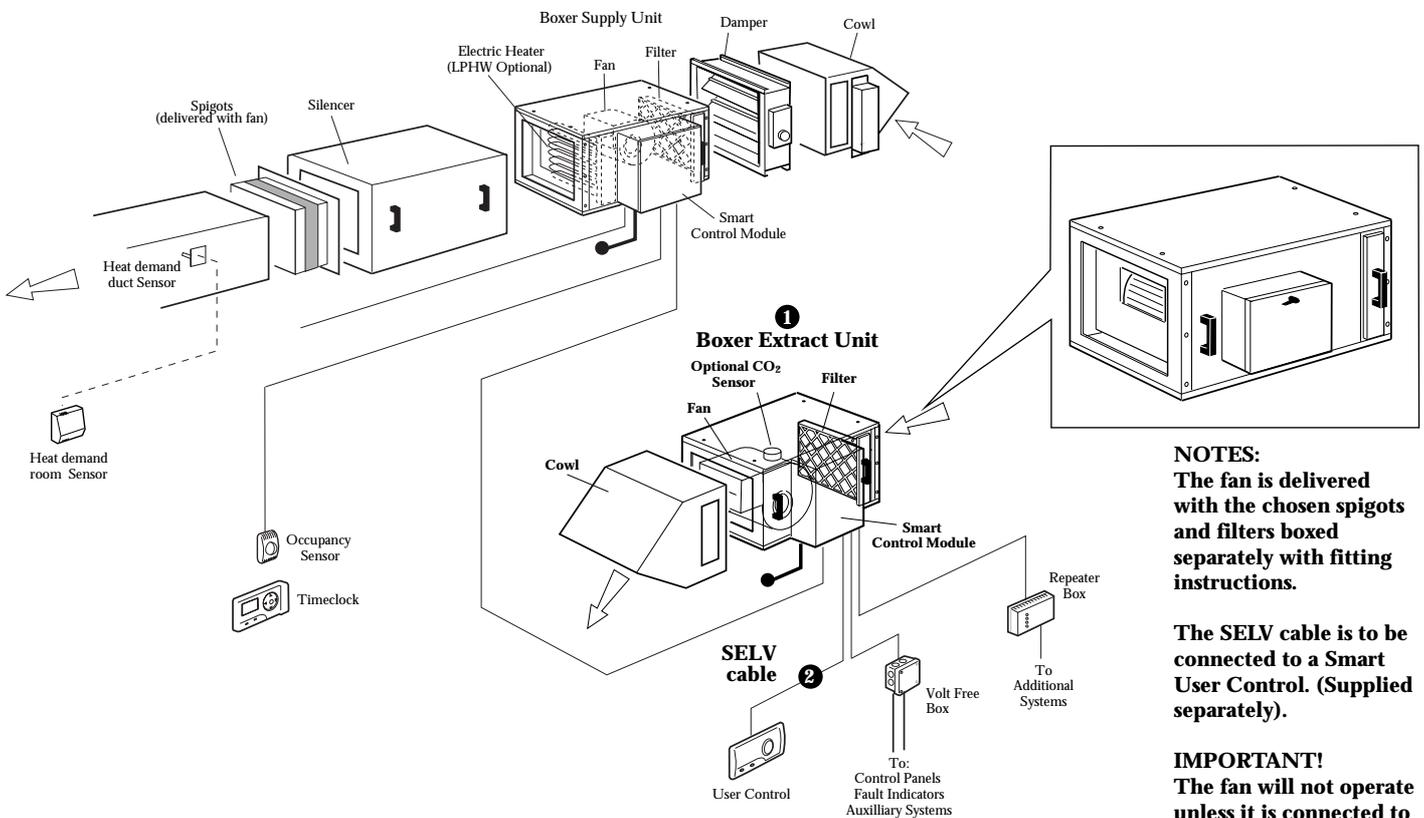
Fig. 1 Typical System, (SBEX Extract unit highlighted).
