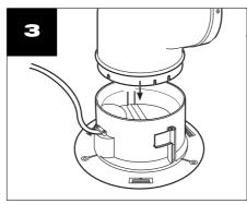
Push the light unit to the  $90^\circ$  bend and click to fit.
