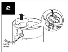
To wire in the light, lift off the cover. Loosen the clamp on the case side. Bring in the two red 12V cables and wire as shown
