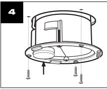
Remove the finisher. Mark and plug three holes using the three fixing holes on the light unit. Secure by using three No. 6 countersunk screws
