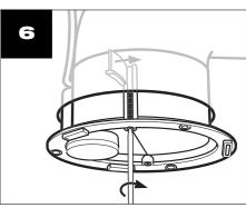
Push the light unit through the ceiling and twist the fingers outwards
