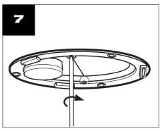
Then tighten the fixing fingers against the ceiling (do not overtighten). To fit the lamp bulb, see details overleaf. Clip on the internal finisher.
