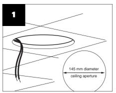
Cut a hole in the ceiling to the size indicated and thread through the two red 12V Power Supply unit cables.
