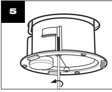
Alternatively, attach the fixing fingers to the light unit using long screws provided
