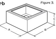
Note: Upper faces of curb are fitted with robust sealing strip.
