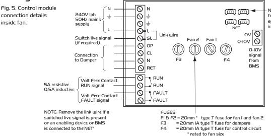
– NET connections for ECOSMART devices eg sensors and inter-connections of fans
