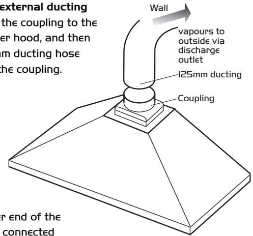
Fig. 6. The other end of the hose should be connected to a discharge outlet that is suitable for cooking vapours and should have a cross section of at least 150cm<sup>2</sup>. The maximum distance between the coupling and the discharge outlet should be 3 metres, with one 90 degree bend.
