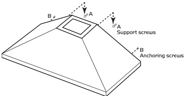
Fully tighten the support screws (A) and then screw the anchoring screws (B) through the relevant holes in the cooker hood into the wall and fully tighten.
