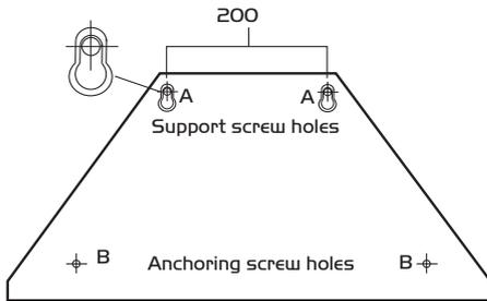
Using a drill bit with a 8mm dia. make holes in the wall on the positions marked.
