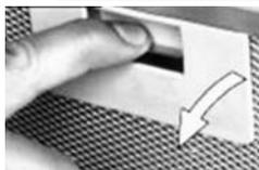
Fig. 10. Remove the grease filters.
