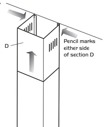
Fig. 8. Take a fixing bracket and place it between the two pencil marks that you made in Fig. 7b.
