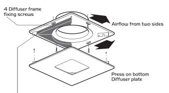
2 Foam strips (supplied) fit on any of the diffuser sides to guide airflow away from a smoke detector and/or obstructions as required.
