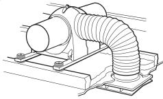
Place anti-vibration mounts (supplied) above and below each batten fixing point and, using the 4 large screws and special washers, fix the unit to the joists.
