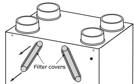
Figure 13. The filters can be removed by pulling on the black tab on the visible end of the filters.
