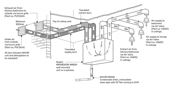
Figure 7b. Typical ducted arrangement for a wall mounted unit using rectangular 204 x 60mm ducting.
