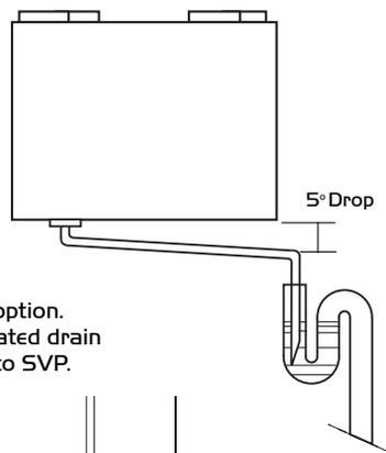
Figure 5b. MVHR-DRAIN option. Condensate drain, uninsulated drain pipe with 10° fall running to SVP.
