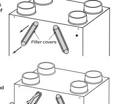
Figure I3.The filters can be removed by pulling on the black tab on the visible end of the filters.
