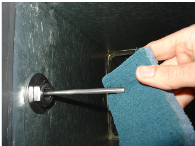
Cleaning of a Cheetah Temperature Sensor, using a scourer.
