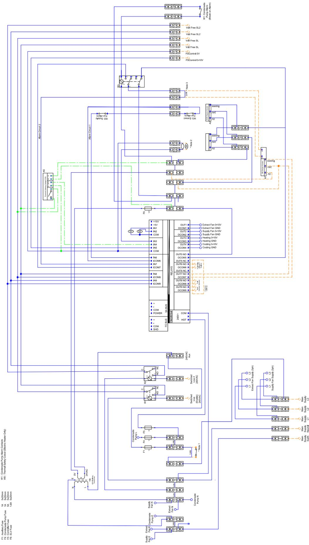
\* Note 1: Emergency shutdown circuit. Break to remove power. Remove link 7, 13 to use.
