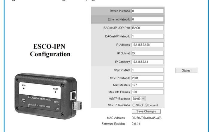
Each parameter of the configuration is explained on the following pages. When *save changes* is selected, the parameters are stored to non-volatile memory and you are prompted to recycle power to the unit.
