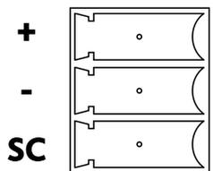
Figure 2. RJ-11 Connector.
