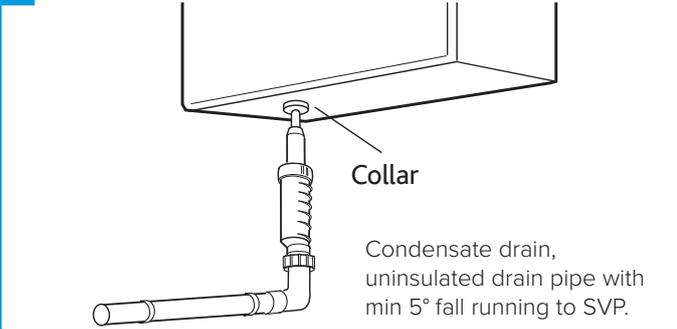
11 "T" Piece CONTRAP & MVHR Drain Connection
