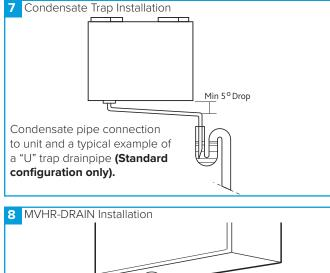
Collar Condensate drain, uninsulated drain pipe with min 5° fall running to SVP.
