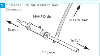
When using a "T" Piece to connect the CONTRAP drainage and the MVHR drain pipework the MVHR drain must always be fitted before the "T" Piece to prevent condensate from feeding back into the MVHR system.
