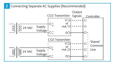
If several sensors share one transformer, the phase (~) must always be the same at each sensor to maintain polarity and avoid a short circuit via a shared common line at the controller, as shown in Figure 3.
