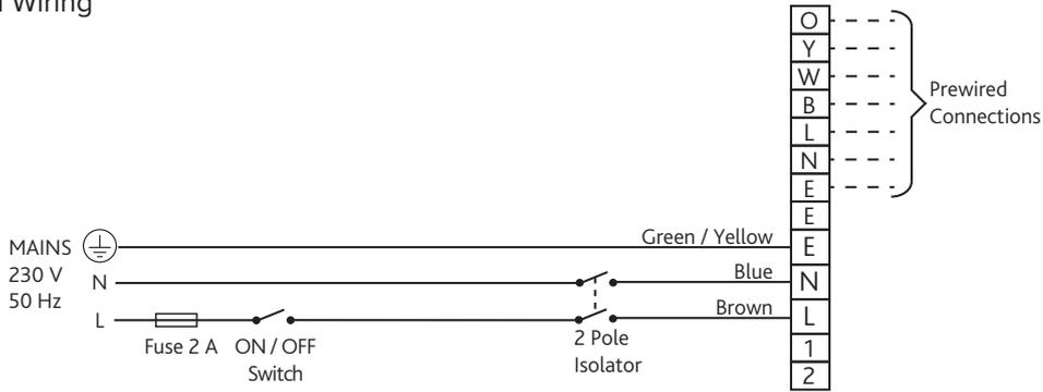
5 Single Speed Wiring with Mains Activated Back-draught Damper
