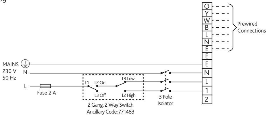
7 Three Speed Continuous Trickle Wiring with Two Boost Speeds
