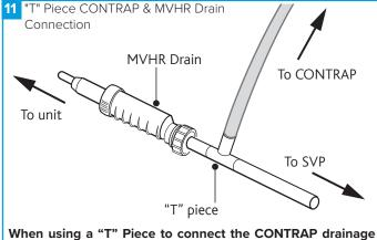
and the MVHR drain pipework the MVHR drain must always be fitted before the "T" Piece to prevent condensate from feeding back into the MVHR system.
