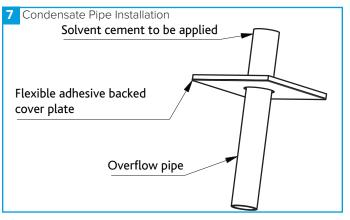
The condensate must be discharged under a water level in a U-trap drainpipe or an alternative drain method which acts as an airlock. This condensate discharge connection is suitable for 21.5mm Ø overflow pipe. Solvent cement should be used to make the joint.
