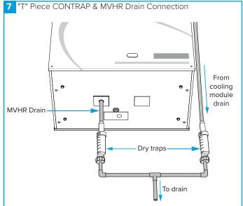
When using a "T" Piece to connect the CONTRAP drainage and the MVHR drain pipework the MVHR drain must always be fitted before the "T" Piece to prevent condensate from feeding back into the MVHR system.
