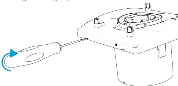
5 Drill Backplate For Recessed Cable Entry
