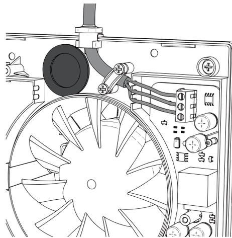
8 Cable Installation For Recessed Cable Entry
