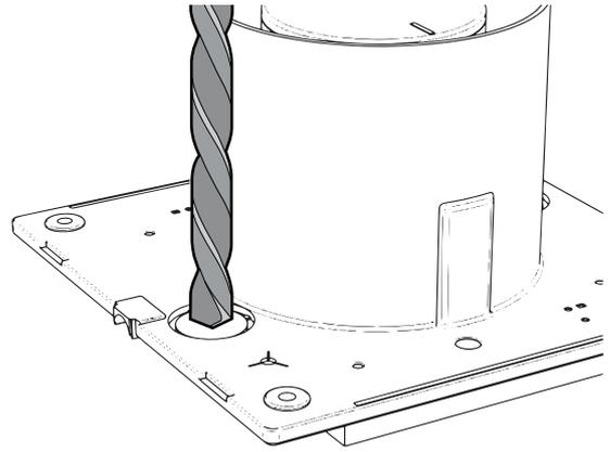
6 Remove Cable Gland For Surface Cable Entry
