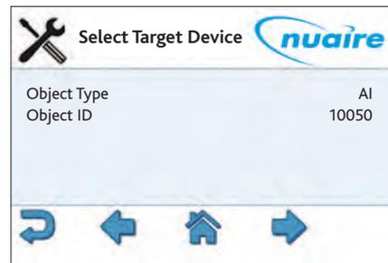
\* This is the setting of the DIP switch on the front of the FAC controller. This can also be discovered by browsing to the network screen while ID is selected in the View Config settings screen.
