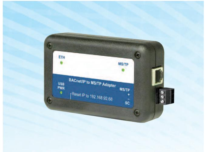
The BACnet router has a USB 2.0, Type B receptacle which is only used to obtain power from a computer or USB adapter. A mains adapter and cable is supplied. The router connects to the FC bus via screwed terminals.
