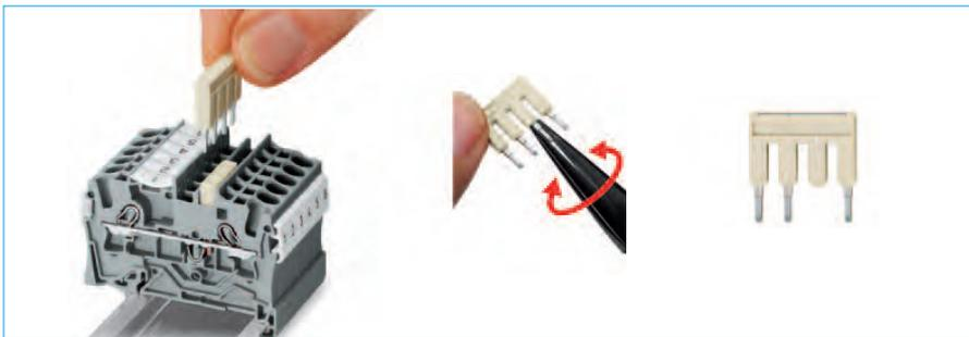
**JUMPER REMOVED** - Insert the operating tool blade between the jumper and the partition wall of the dual jumper slots, then lift up the jumper.
