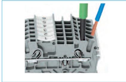
**CONDUCTOR REMOVAL** - Insert an operating tool in to the operating slot to remove the conductor, just like the original CAGE CLAMP® terminal blocks.
