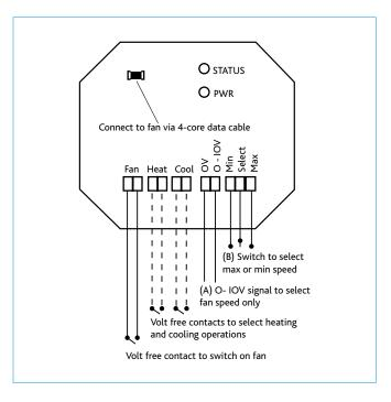
As the room  ${\rm CO_2}$  and temperature rises, the fan speed will progressively increase in steps until the upper threshold values are reached. When both  ${\rm CO_2}$  and temperature readings are in operation, whichever reading that results in higher fan speed will be used by the fan unit.
