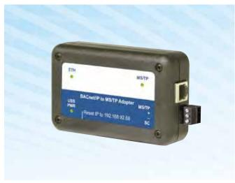
The BACnet router has a USB 2.0, Type B receptacle which is only used to obtain power from a computer or USB adapter. A mains adapter and cable is supplied. The router connects to the FC bus via screwed terminals.
