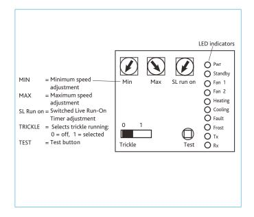
The Ecosmart control module has the following two options fitted as standard.
