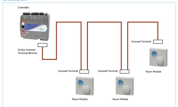
Cable type: Plain-ended shielded 2 twisted pair 22AWG
