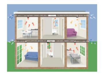
During the warmer months to provide you with cooler air, the system is set to bypass the heat exchanger. This means the air pulled in from outside will not be tempered as it does not use the heat that the heat exchanger has recovered from your home.
